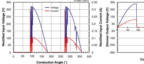
Figure 10. Example of Phase Angle Dimmer Showing Erratic Firing.
