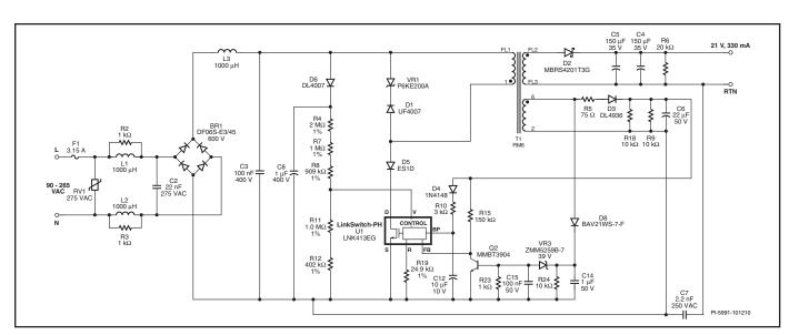
Figure 8. Schematic of an Isolated, Non-Dimmable, High Power Factor, Universal Input, 7 W LED Driver.
