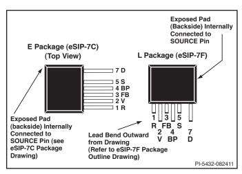
Figure 4. Pin Configuration.
