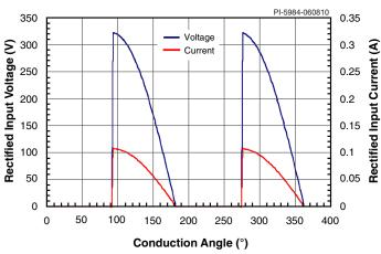
Figure 9. (a) Ideal Input Voltage and Current Waveforms for a Leading Edge TRIAC Dimmer at 90° Conduction Angle. (b) Resultant Waveforms Following Rectification of TRIAC Dimmer Output.
