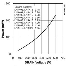
Figure 15. Power vs. Drain Voltage.
