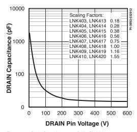
Figure 14. Drain Capacitance vs. Drain Pin Voltage.
