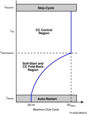
Figure 5. FEEDBACK Pin Current Characteristic.
