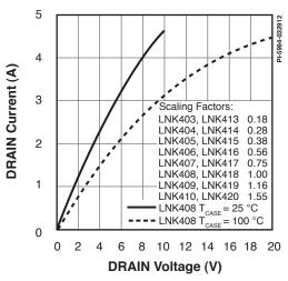
Figure 16. Drain Current vs. Drain Voltage.
