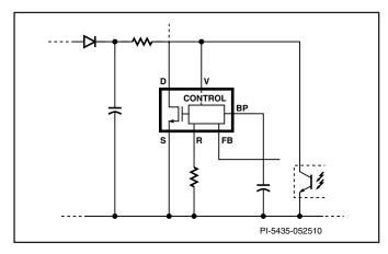
Figure 6. Remote ON/OFF VOLTAGE MONITOR pin Control
