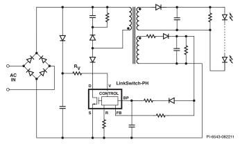
Figure 1. Typical Application Schematic.
