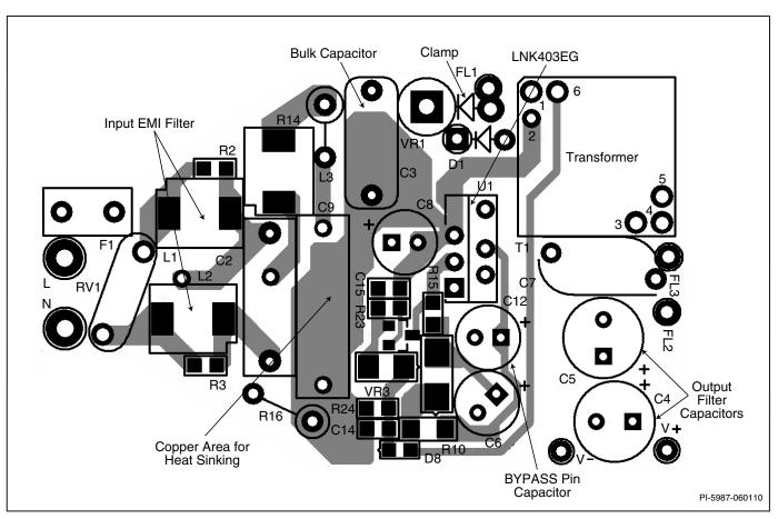
Figure 12. RD-193 7 W Layout Example, Top Layer.
