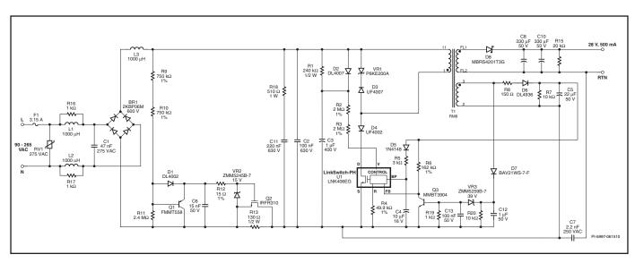
Figure 7. Schematic of an Isolated, TRIAC Dimmable, High Power Factor, Universal Input, 14 W LED Driver.
