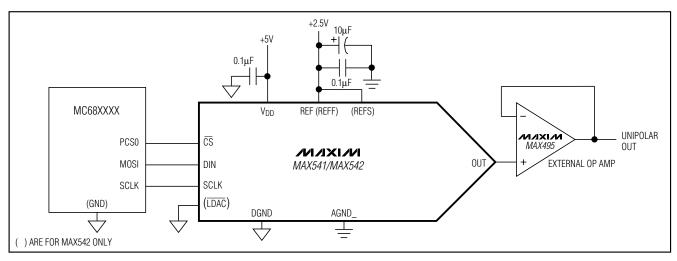
Figure 2a. Typical Operating Circuit—Unipolar Output
