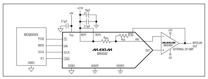
Figure 2b. Typical Operating Circuit—Bipolar Output
