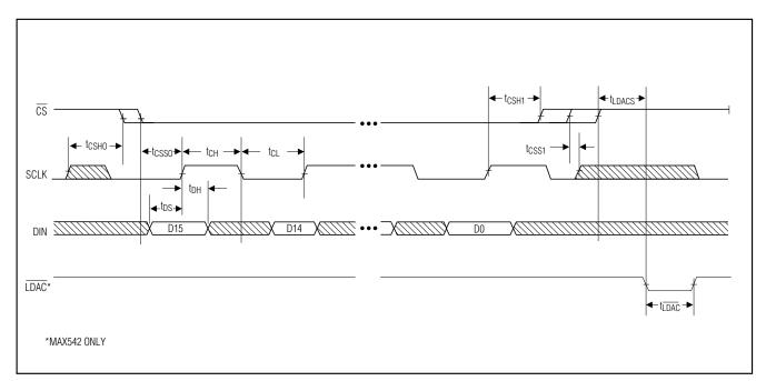
Figure 1. Timing Diagram
