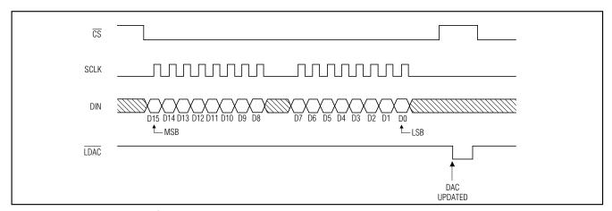
Figure 3b. MAX542 4-Wire Interface Timing Diagram
