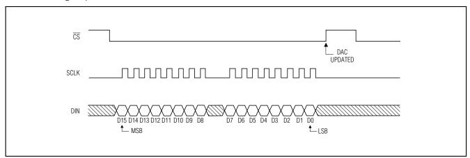
Figure 3a. MAX541/MAX542 3-Wire Interface Timing Diagram (LDAC = DGND for MAX542)
