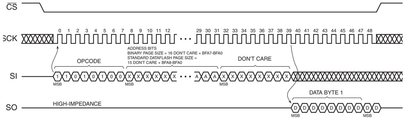
Figure 19-6. Buffer Read (Low Frequency: Opcode D1H)
