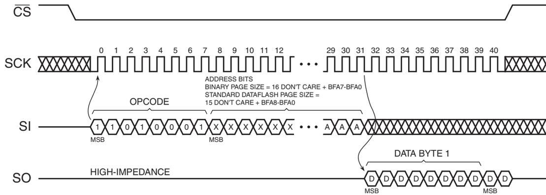
Figure 19-7. Read Sector Protection Register (Opcode 32H)
