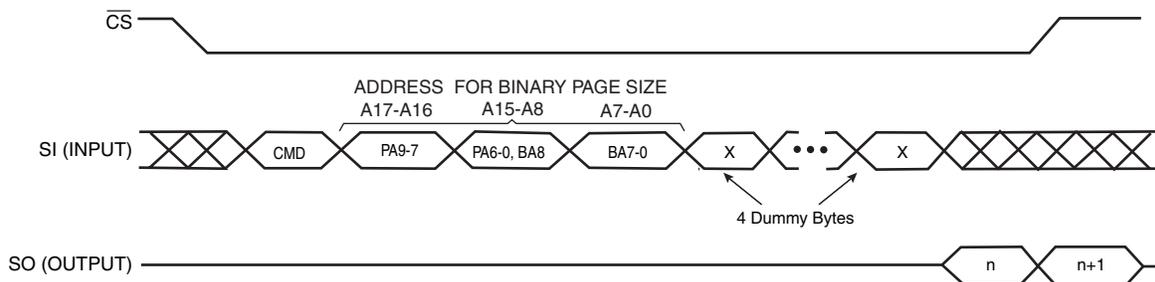
Figure 18-2. Main Memory Page to Buffer Transfer (Data from Flash Page Read into Buffer)
