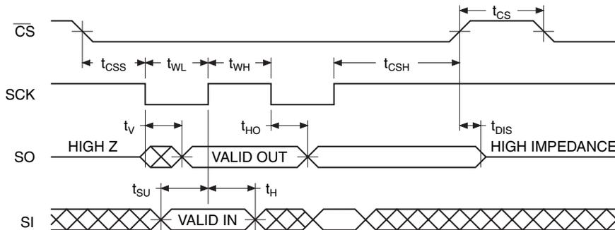
Figure 17-3. Waveform 3 – RapidS Mode 0 ( $F_{MAX} = 66\text{MHz}$ )
