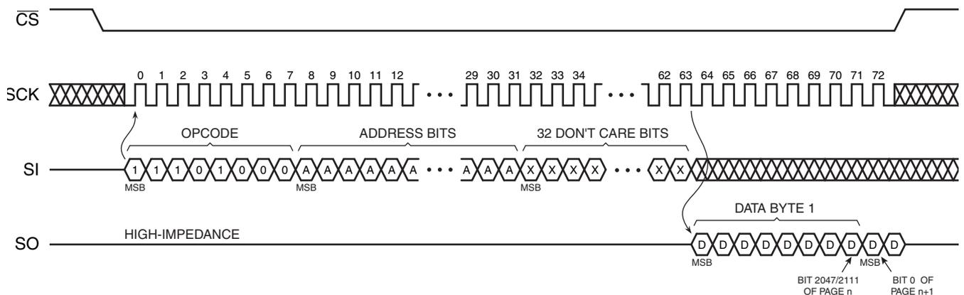
Figure 19-2. Continuous Array Read (Opcode 0BH)
