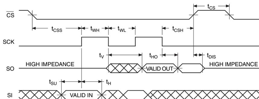
Figure 17-4. Waveform 4 – RapidS Mode 3 ( $F_{MAX} = 66\text{MHz}$ )
