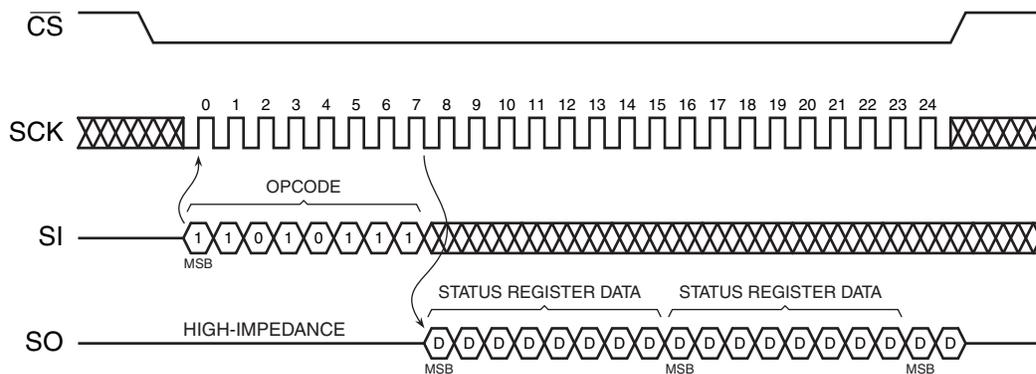
Figure 19-11. Manufacturer and Device Read (Opcode 9FH)
