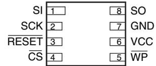
Notes: 1. The metal pad on the bottom of the UDFN package is floating. This pad can be a “No Connect” or connected to GND
