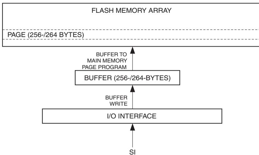
Figure 17-10. Buffer Write
