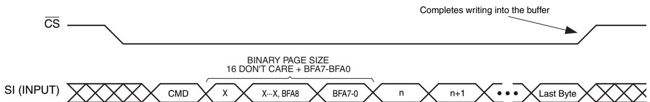
Figure 17-11. Buffer to Main Memory Page Program (Data from Buffer Programmed into Flash Page)
