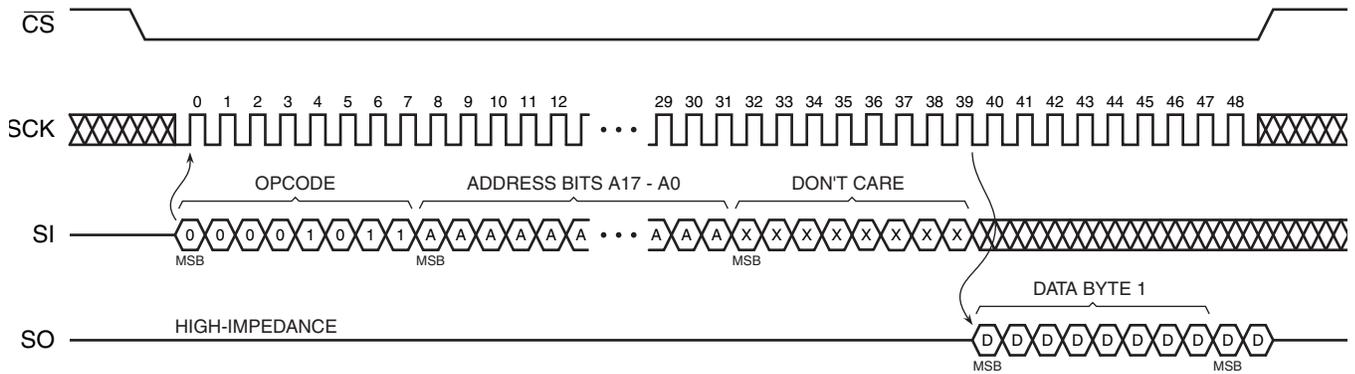
Figure 19-3. Continuous Array Read (Low Frequency: Opcode 03H)
