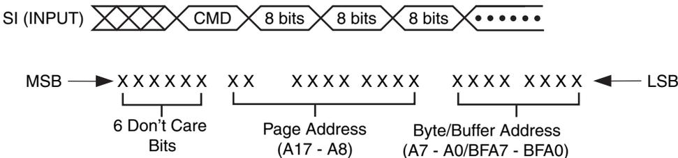
Figure 17-8. Command Sequence for Read/Write Operations for Page Size 264-Bytes (Except Status Register Read, Manufacturer and Device ID Read)
