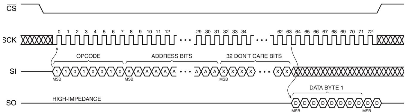
Figure 19-5. Buffer Read (Opcode D4H)
