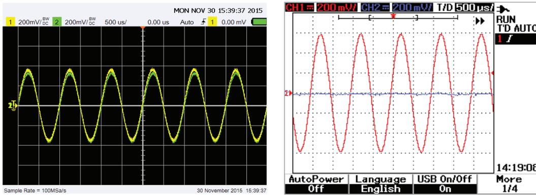
Figure 3. Two different floating measurement waveforms captured with an oscilloscope with channel-to-channel isolation (left) and an oscilloscope without channel-to-channel isolation (right)
