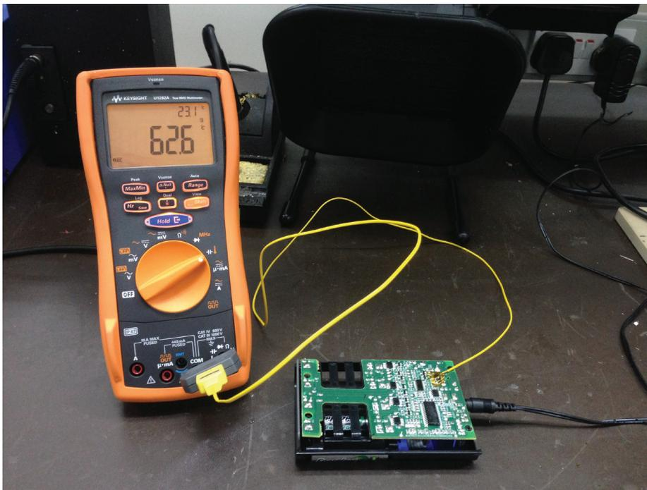
Figure 2. Monitoring the temperature of a circuit board with the U1282A handheld digital multimeter
